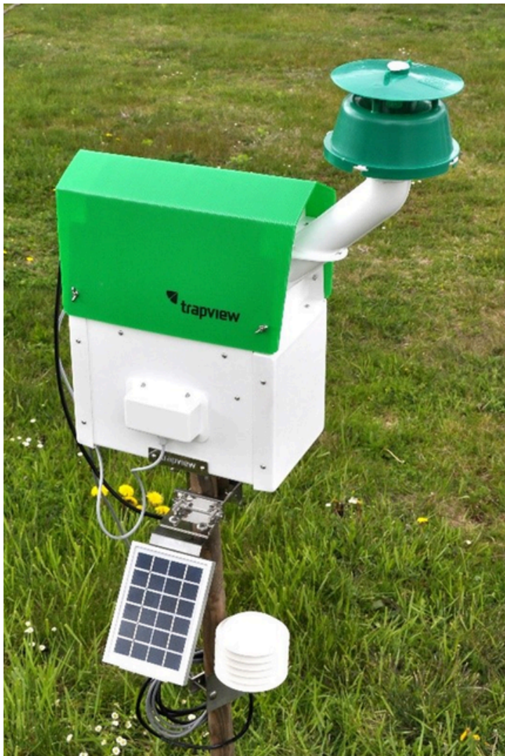
A solar-powered monitoring device for tracking pest populations
